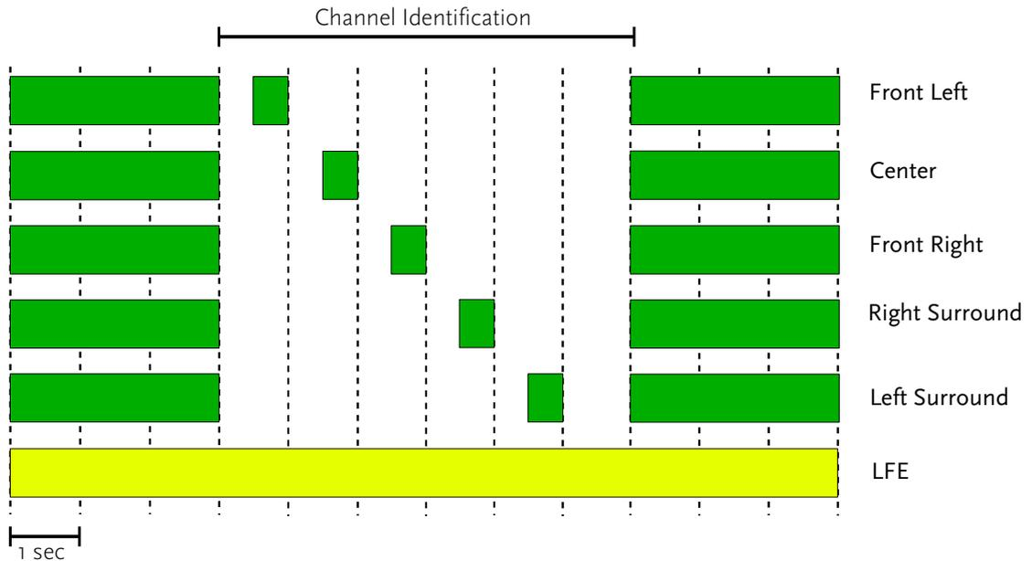
The channel identification will adapt to the kind of used surround, from which total length we understand how many channels we are using: 5.0; 6.0; 5.1; 7.0; 7.1 and so on.
