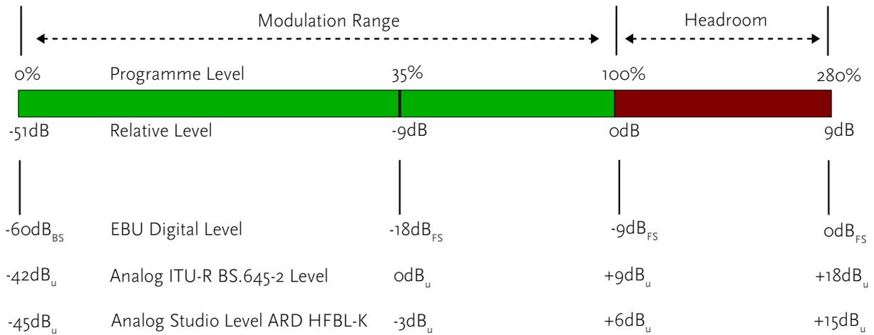
Considering the scale settings, the “full scale” (100%; 0dB) like the specified “Headroom” should match the “Attack Time” and “Release Time” of the relative Programme Meter. For instance the VU-Meter that can be considered relatively slow, obviously need an appropriate Headroom due to the invisible signal peak. Consequently the difference between 100% and the aligning level need to be smaller than other considered.
