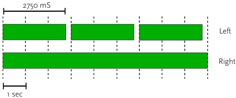
The interruption make possible to hear the phase realtions and to identify the mono mix.
